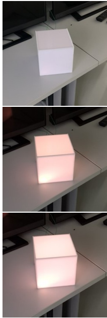
Figure 2: When a user has a weak focus, calmworklight is pulsing from low (1) to a higher (2, 3) light emission.
